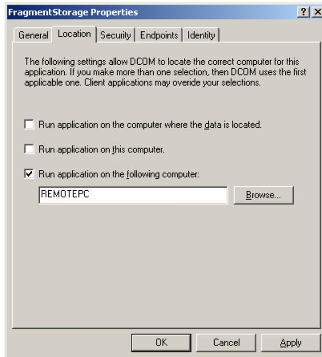
Figure 44. Remote computer selection for the FragmentStorage service
