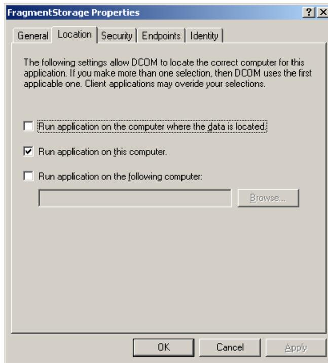
**Figure 45. Local computer selection for the FragmentStorage service**
