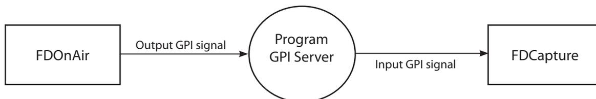
SoftGPI signals are configured by user in the SLGPISoftConfig application, which is a part of the ForwardT Software Set.
