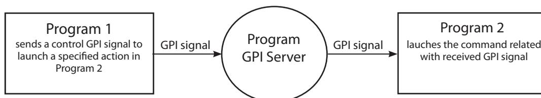
For transferring a control signal from one program to another a pair of GPI signals (input and output) is used:
