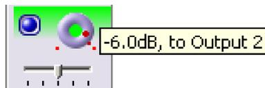
Tool tip about the input signal volume level at transmission to the output channel
